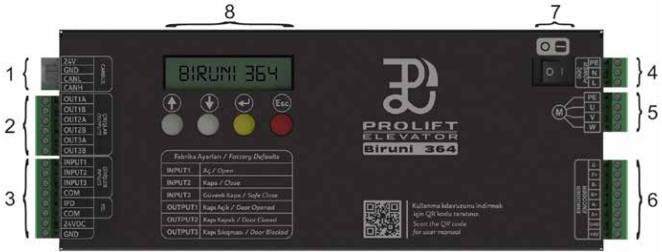
Figure 1 Door Controller Internal Structure
